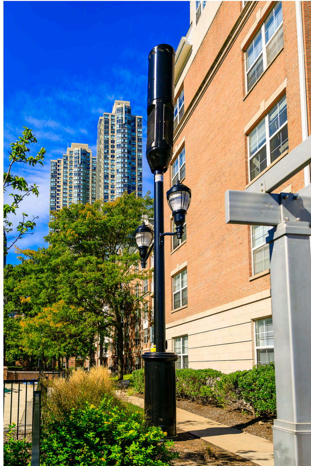
Telecom Enhanced Decorative (TED) Light Poles are the perfect way to adapt communications and smart city requirements into traditional lighting structures.
